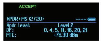
The 20-character 4-line display provides for easily viewable data and parametric measurements as required for Mode S Elementary and Enhanced Surveillance testing. For legacy test modes, the menu structure and displayed data format have been retained so that minimal changes are required of fielded procedures.
